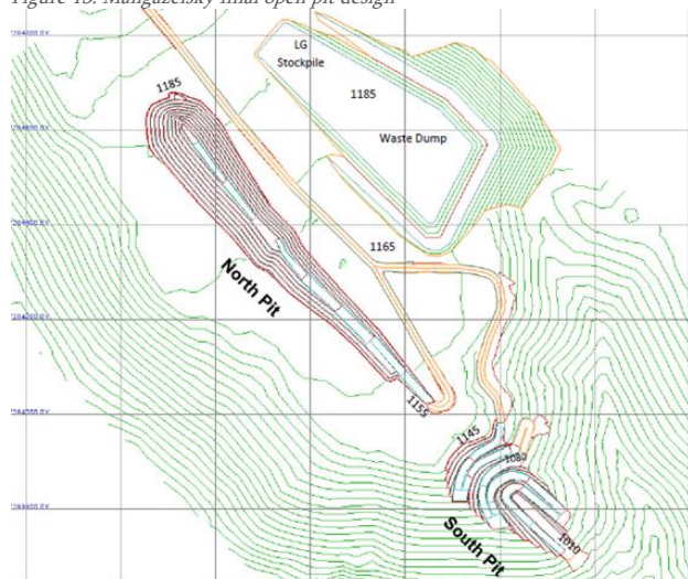
Figure 13: Mangazeisky final open pit design
